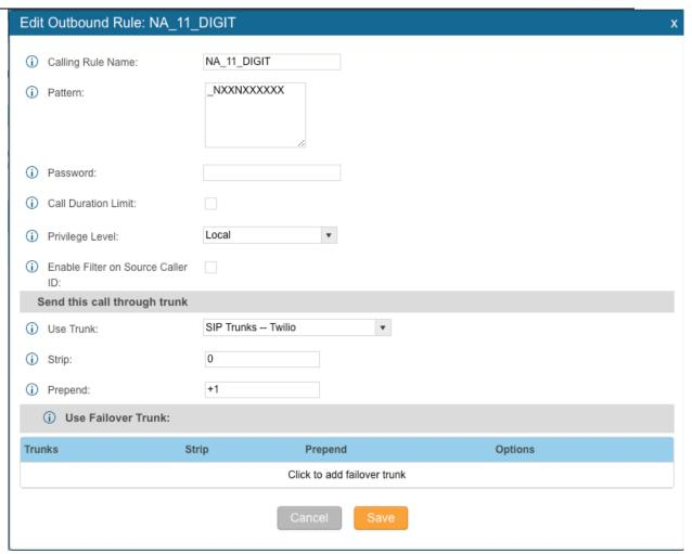
Please note: Twilio only supports E.164-formated. Therefore, please prepend "+1" to the calls that have been placed on current trunk. SIP Register Trunk is used to support outbound calls, therefore, outbound rules are not required for rest of the 4 SIP Peer Trunks since they are used for taking inbound calls.
