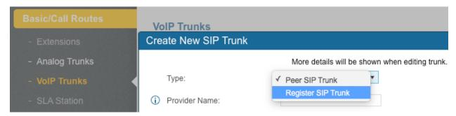
In the following dialog, configure the elements circled in yellow which include - **Host Name**, **Username**, **Password**. You can also add a Provider name like Twilio. Please make sure that **Keep Trunk CID** is enabled in order to match authentication credential on Twilio.
